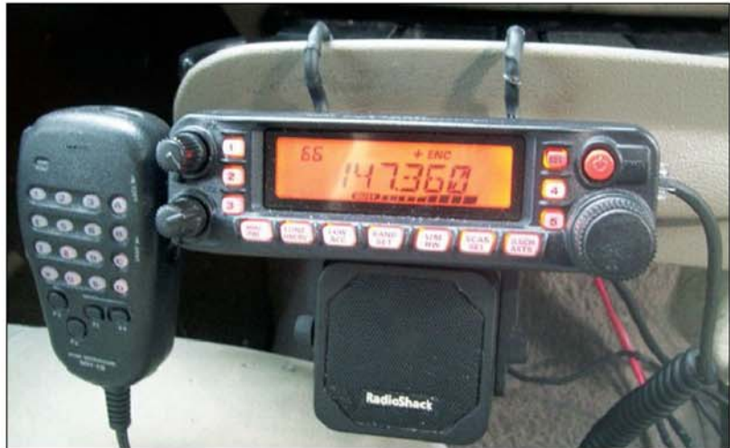
Figure 1 — The transceiver's control head is hung from the front of the drawer that contains cup holders and an ash tray.
