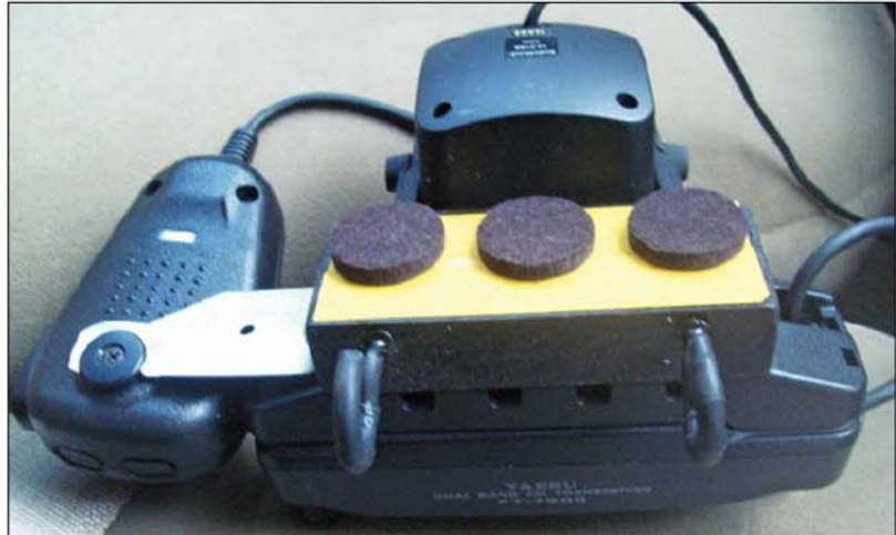
Figure 2 — Rear view of wooden mounting block for the transceiver's control head. The cup hooks for hanging the block are covered with heat-shrink tubing and the three stick-on felt pads dampen vibration as well as protect the finish of the drawer front where the block is hung. The microphone hook is shop-fashioned from a metal mending plate.
